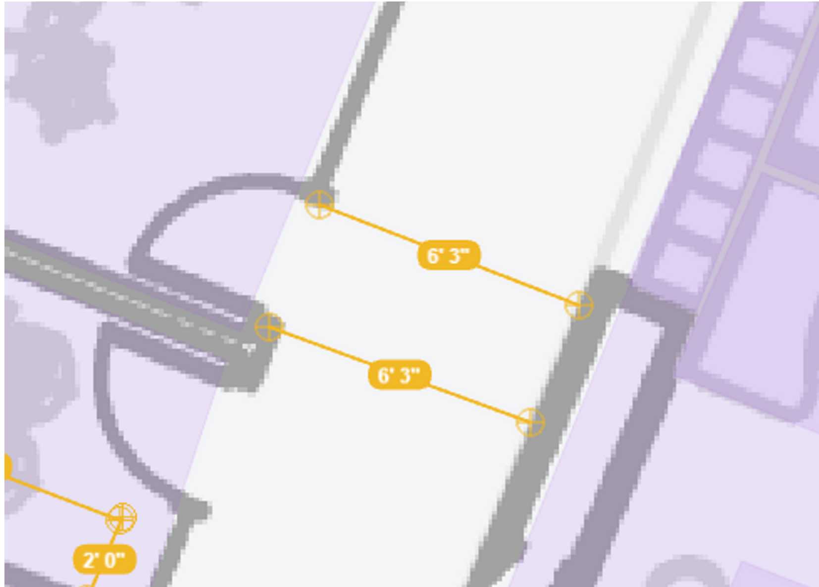
This door has the necessary clearance for Entry LR mounting
